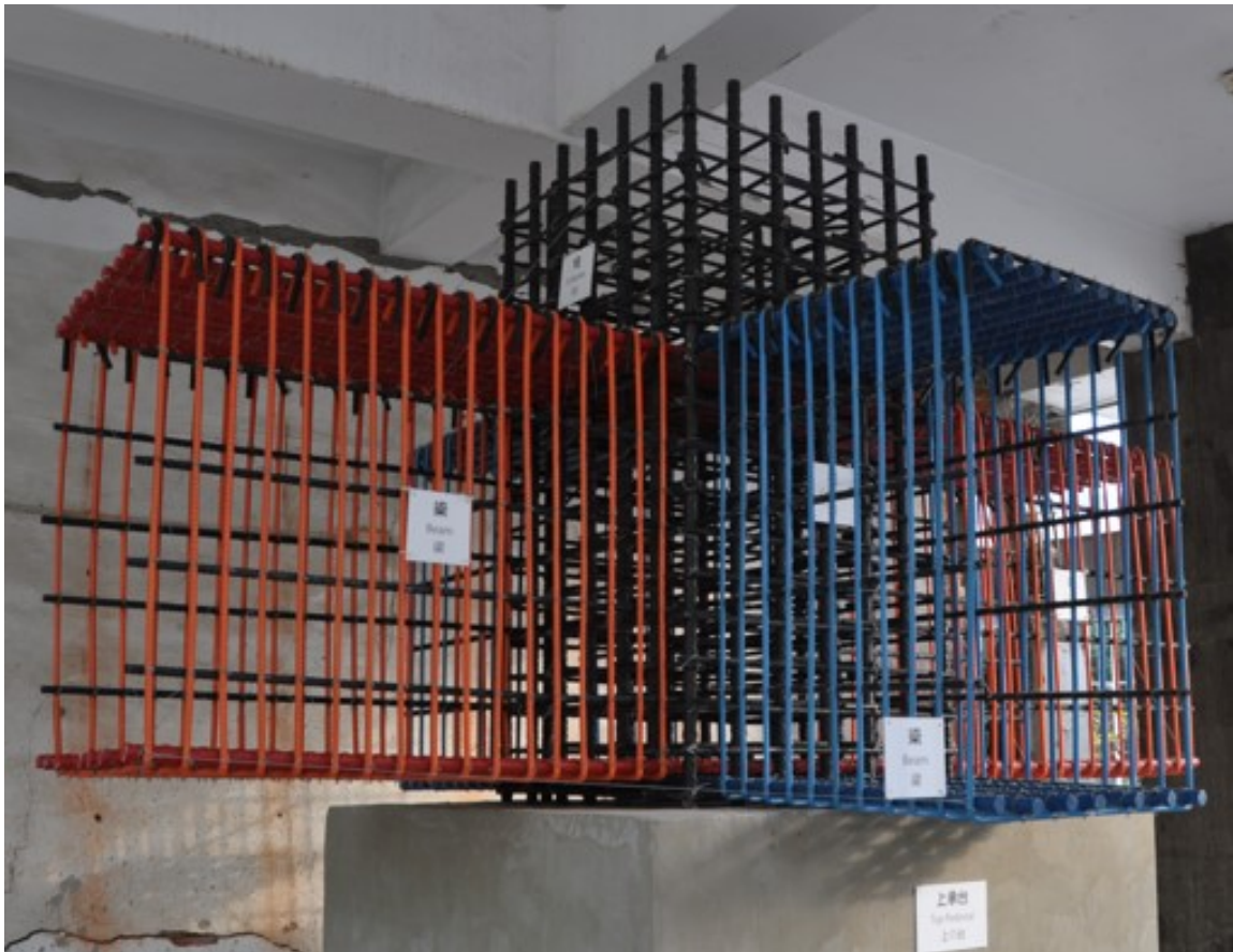
Figure 8. Excessive cross-sectional area and steel reinforcement resulting from the revised seismic design code after the 921 Jiji earthquake (Lin et al. , 2022).
